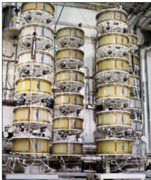
**Figure 2.** The “Stack” column used for insulin purification in the 1970s. Single sections of this column became standard in the pilot scale use of ion exchangers for, for example, plasma protein purification. The 16-cm bed height was a driving force in the move to short bed columns and the scale up to a 30 cm x 150 cm bed column as standard in the 1970s.
